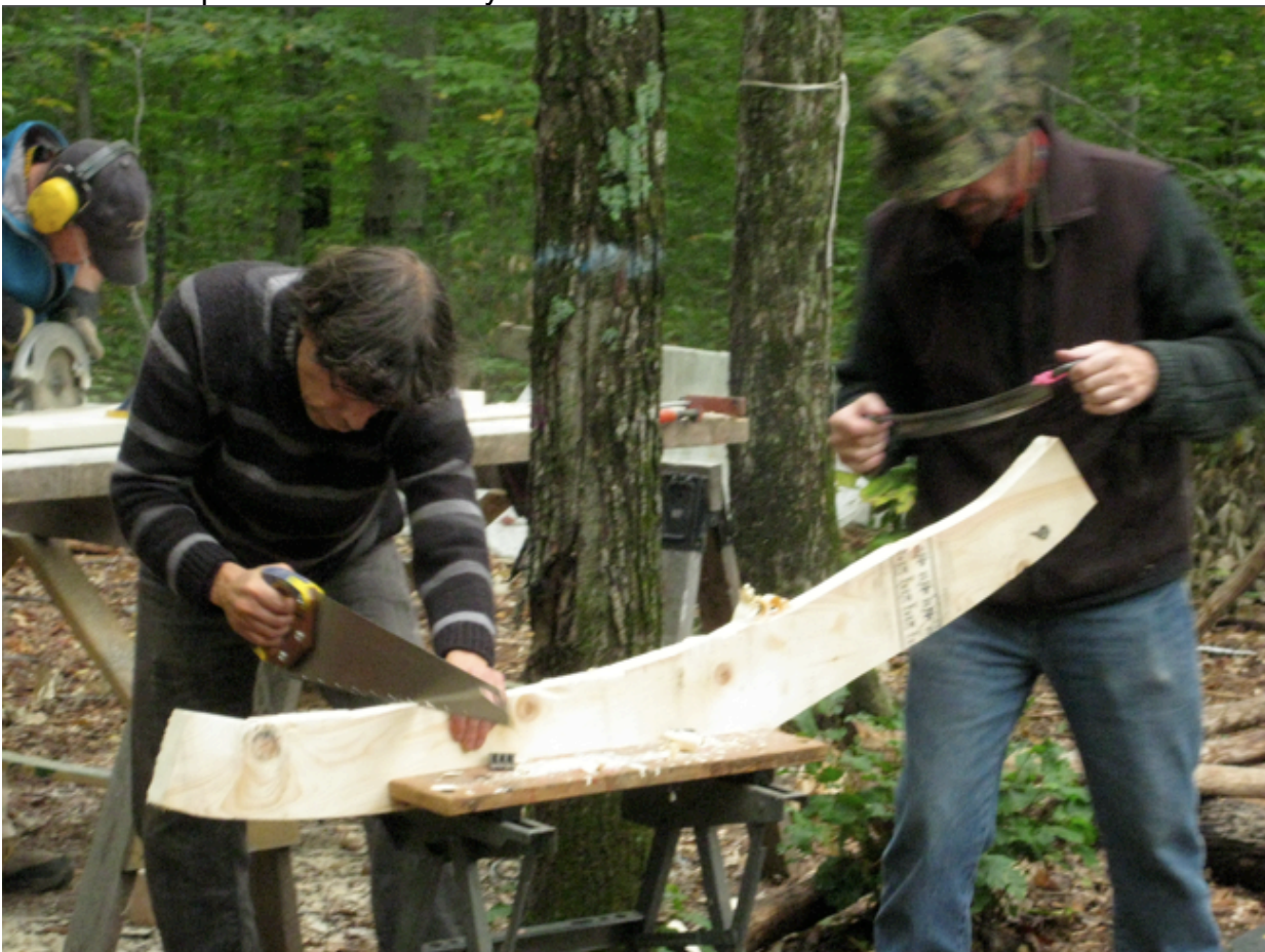
We had to plane and chisel to achieve the correct curve in each piece of the rib.
